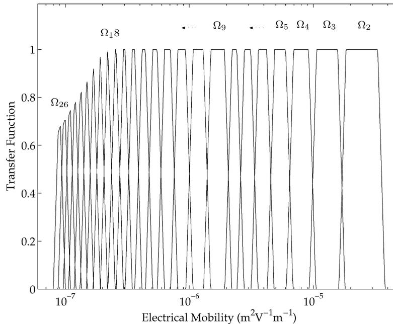
FIG. 8. Non-diffusing transfer function of the DMS classifier. The instrument's settings used for the calculations are:  $V_L = 9910$  V,  $Q_a = 5$  l  $\text{min}^{-1}$ ,  $Q_s = 35$  l  $\text{min}^{-1}$ , and  $P = 250$  mbar.
