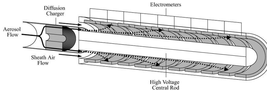
FIG. 1. Schematic layout of the Differential Mobility Spectrometer (DMS).
