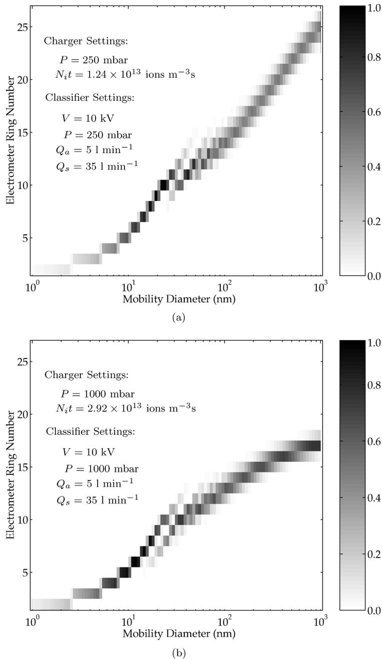
FIG. 10. Kernel of the instrument at (a) subatmospheric and (b) atmospheric pressures. Both kernels are estimated using Fuchs' limiting sphere theory and the non-diffusing transfer function (Equation 23).
