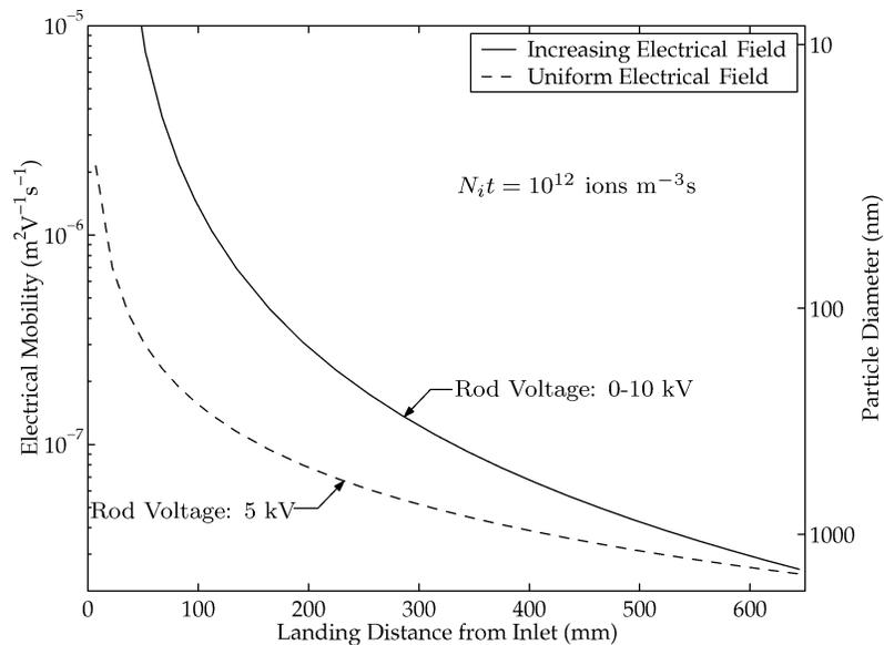
FIG. 3. Comparison of the mobility and size of the particles collected along the DMS column when a uniform or a linearly increasing voltage is applied on the central rod. The correlation between particle diameter and mobility is made using Fuchs' limiting sphere theory at atmospheric conditions with an  $N_i t$  parameter, as indicated in the figure.
