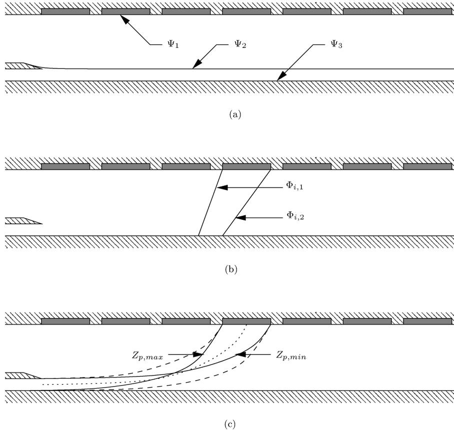
FIG. 6. Schematic diagram of (a) the fluid streamlines, (b) the electric field lines, and (c) the particle streamlines in the classification column.
