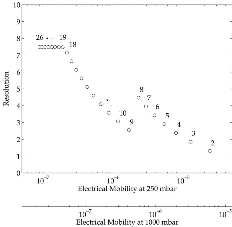
FIG. 9. Electrical mobility resolution of the DMS classifier. The results are obtained using Equation 6 to estimate the midpoint mobility diameter for every channel and the non-diffusing transfer function (Equation 23) to estimate the full width at the half maximum.
