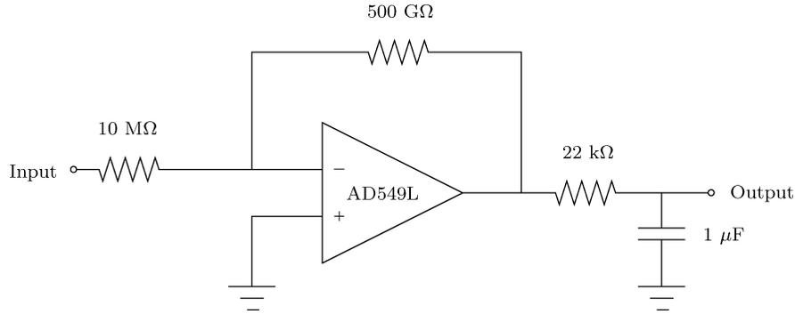
FIG. 5. Schematic diagram of the electrometer circuit of the DMS.
