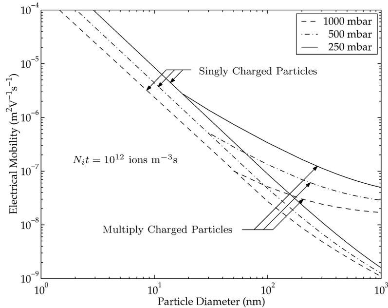
FIG. 2. Electrical mobility of unipolarly charged particles at different pressures. All calculations are performed using Fuchs' limiting sphere theory and keeping the rest of the conditions unchanged.
