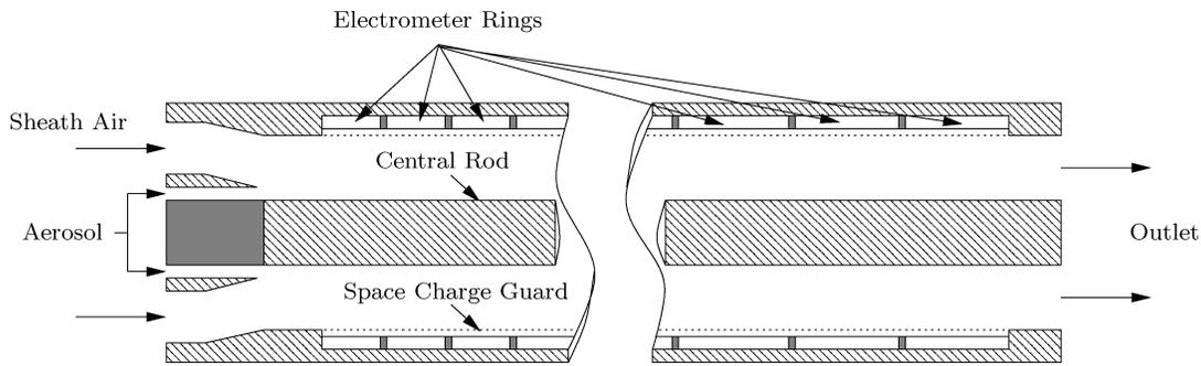
FIG. 4. Schematic diagram of the classification column of the DMS.
