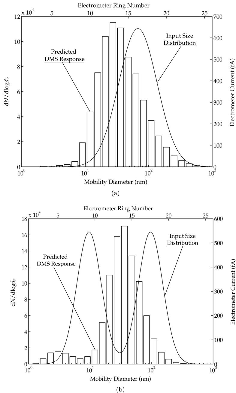
FIG. 11. Response of the instrument on different aerosol size distributions. The solid lines represent the input size distributions of the sample aerosol and refer to the left and bottom axes, while the bar plots correspond to the response of the instrument (currents on every channel) and refer to the right and top axes of the graphs. The predicted electrometer readings are based on the non-diffusing kernel at 250 mbar (Figure 10a).
